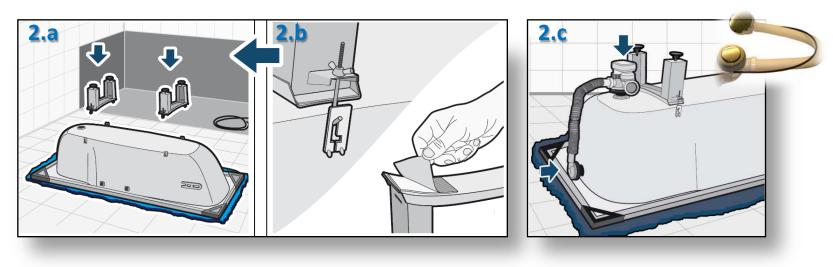
2. Install the bathtub feet and waste valve according to supplied instructions.
