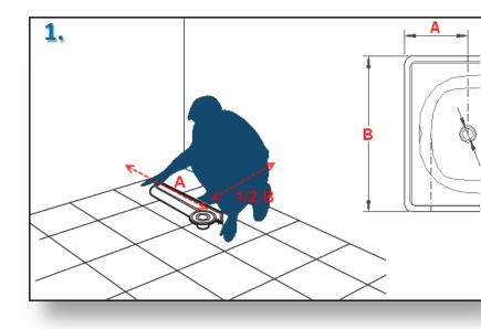
1. Before starting installation of the bathtub be sure to properly prepare the waste pipe
