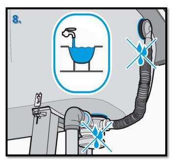
8. Once the connections are completed fill the bathtub with water, wait for about 2 hours and check for water leaks.
